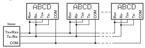
Below shown control via RS485 4-wire bus (optional four-wire Modbus definition) is optionally possible.
