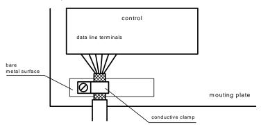
The cable shielding is to be connected at both cable ends. If equipotential bonding currents are expected due to the cable arrangement, electrical isolation is to be performed on one side. In this case, capacitive connection (approx. 0.1µF/600 V AC) of the shielding on the isolated side must occur.
